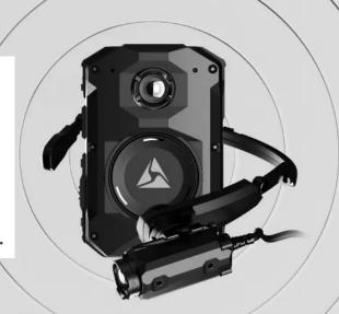
Officers no longer need to decide between using chest mounted cameras or flexible POV modules, as the Axon Body 4 has the option to add on a quick connecting POV camera with the Flex POV module.
